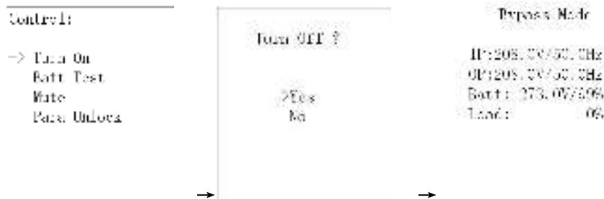
NOTE: You may simply turn off UPS by pressing "OFF/ESC" button in home page. It's not necessary to enter control menu to turn off the UPS.
