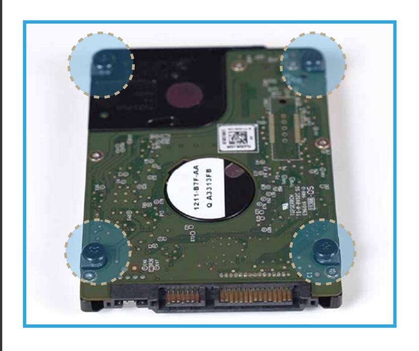
ii. Install the 2.5" HDD screws on your SSD screw holes.
