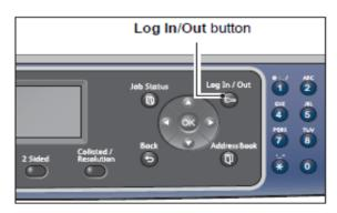
2. Enter passcode using the numeric keypad and press **OK** button Passcode is initially set to "1111"
