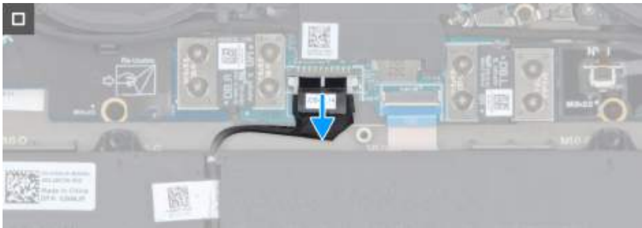
Obrázek 16. Disconnect the battery cable from the system board
