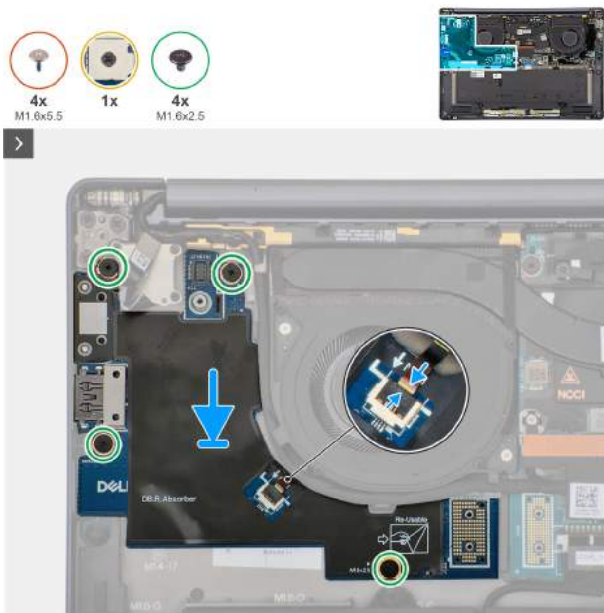
Obrázek 45. Installing the right I/O board (without WWAN antennas)
