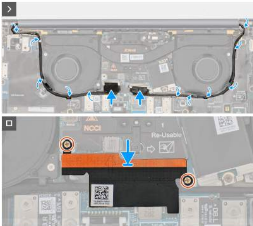
Obrázek 63. Connecting the display and camera cables
