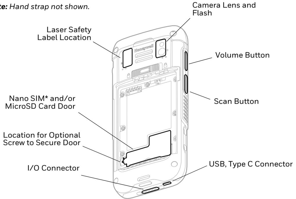
\* Cellular phone feature is available only on WWAN models (CT47X1N). The SIM slot supports use of an UICC card for NFC Secure Element NFC link encryption.
