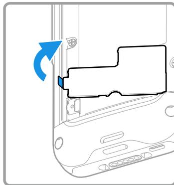
6. Insert the microSD card into the SD card socket.
