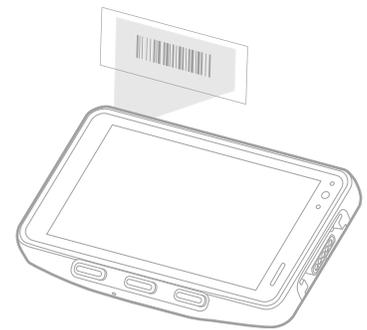
**Note:** *In the Scan Demo app, not all barcode symbologies are enabled by default. If a barcode does not scan, the correct symbology may not be enabled.*
