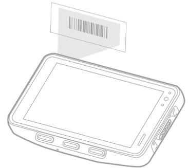
**Note:** *Not all barcode symbologies are enabled by default. If a barcode does not scan, the correct symbology may not be enabled.*
