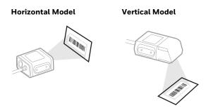
**Note:** If the light level in the room is not high enough, the barcode may not be read. If room lighting is not sufficient, auxiliary lighting may improve scanning performance
